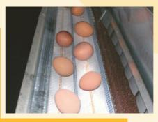
The lift system provides less crack eggs and safe collection. The Poly Propylene belts (PP, 250 mm. wide) bring the eggs from nest system and the reel conveyors transport the egg to the packing room.
