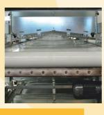
Manure removal system consists mainly of a PP (Poly Propylene) conveyor belt, which runs underneath the cage, a drive unit with rollers, belt supports and guides. Manure removal system facilitates automatic collection and removal of manure and can be built as long as 150 m. Galvanized material used in the entire system provides corrosion resistance while ensuring a long operational life.
