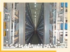
A specially designed lift system ensures crack-free eggs while providing easy egg collection. PP (Poly Propylene) conveyor belts collect the eggs from cage and the eggs are transported to the packing room via reel conveyors.
